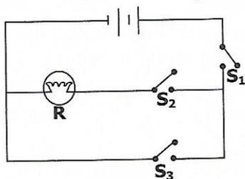
Which switch(es) must be closed to make bulb **R** to light?
